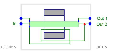
Ferrite bead as a transformer core
