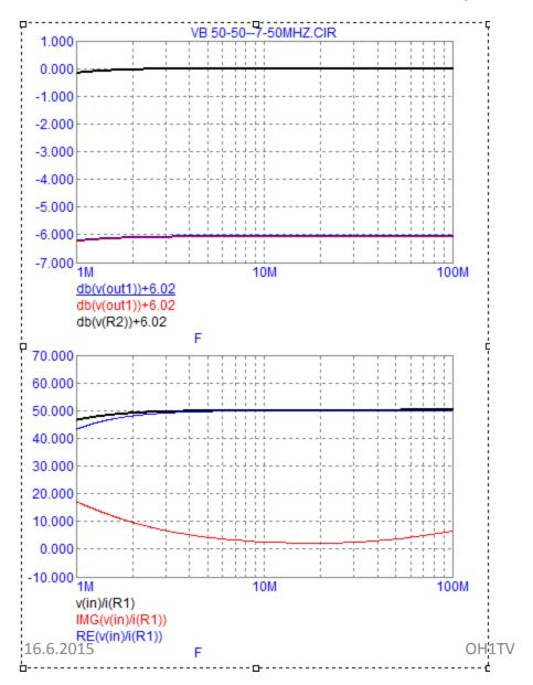
Black = attenuation to load R2 Red = voltage level against ground at Out1 Blue = voltage level against ground at Out2
