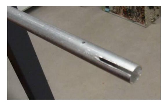
Angle grinder is used to cut about 2mm wide and 30mm long slot Hole for screw is dia 3mm
