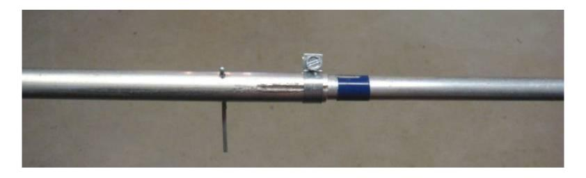
Hose clamp is needed to make good contact between the parts. M3 screw or split pin alone is not enough on 50MHz. Clamps marked 11mm seem to work best for 12mm tube.
